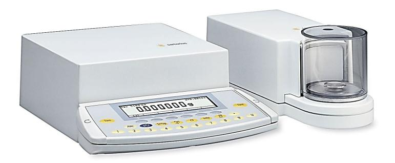
Capacity x Readability (grams x μg): 5.1 g x 1 μg Repeatability, micrograms (standard deviation) ± 1 μg Linearity, micrograms: ± 4 μg Linearity: 0-500micrograms±2μg
