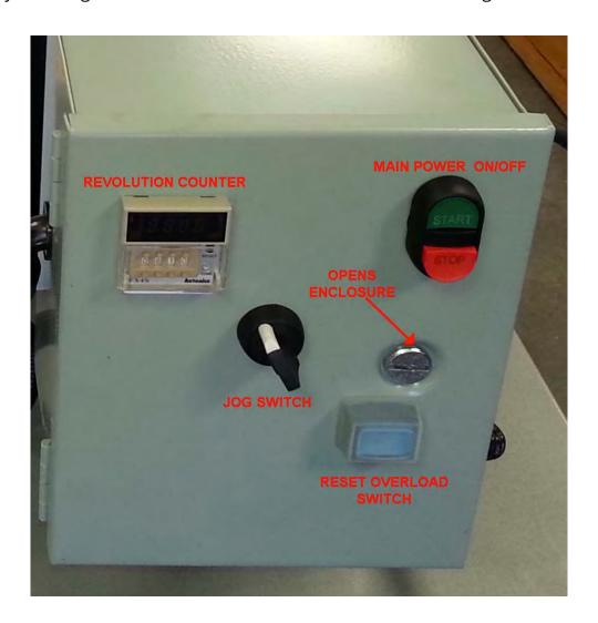
To set the revolution counter, refer to the photo below. By pushing the bottom row buttons, the counter number is increased. Pushing the top row of buttons decreases the counter number. The actual revolutions is displayed in the digital led display. Then the digital display reached the number input below, the mill shuts off.
