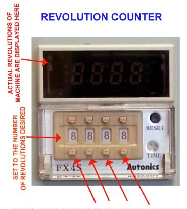
PRESS LOWER BUTTONS TO SET NUMBERS ABOVE THEM THE BOTTOM BUTTONS MOVE NUMBER HIGHER THE TOP BUTTONS MOVE THE NUMBER LOWER
