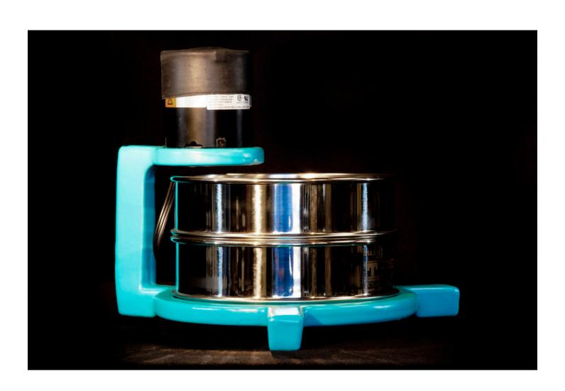
The Sepor Wet-Dry Sieve Shaker is supplied for the purpose of conducting relatively simple size analysis for materials. The sieve shaker uses standard 8 inch diameter laboratory sieve screens and has a capacity for 2 full height 8" diameter sieve screens. The smallest opening sieve screen that should be used with the Wet-Dry Sieve Shaker is 100 mesh.
