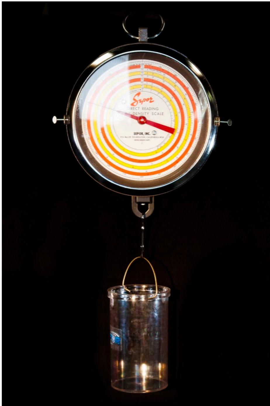
**Mounting:** A 2-1/2" diameter supporting ring provides the method of hanging the scale mechanism freely in space.
