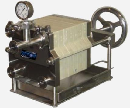
Results from this little lab plate and frame filter can be used to size process filters, and determine the number and quantity required to filter large volumes of slurry. Plate and frame filters can be coated with diatomaceous earth, and used to filter very low solids and or particle size slurries.
