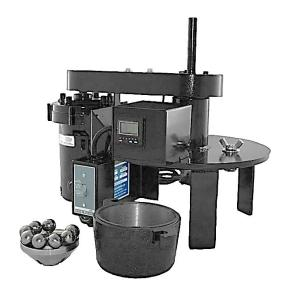
The Hardgrove Tester gives reproducible results because the work done on the sample is so closely controlled. Since the sample is always in the path of the rolling balls, the energy is evenly distributed throughout the sample. The Hardgrove Grindability Tester is simple and clean operating. No sample is lost as the pulverizing takes place in a closed compartment. After releasing the lower portion of the grinding unit by the 2 thumbscrews, it can be removed and cleaned with a brush.
