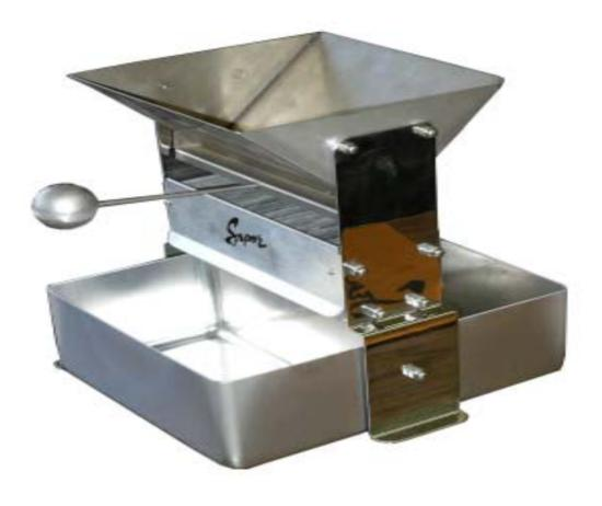
Prior to splitting material, it is good practice to mix the sample by repetitive dividing and recombining the entire sample several times.
