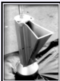
Replaceable Vezin Sample Cutter
