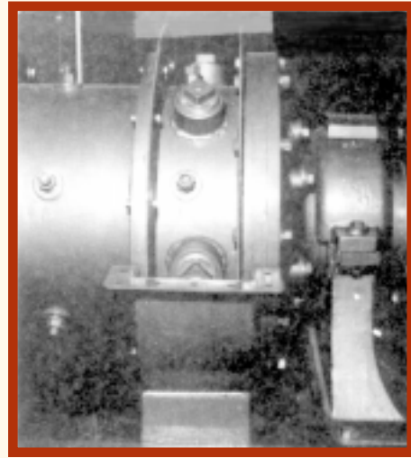
Optional Peripheral Discharge Arrangement (Cover Removed)
