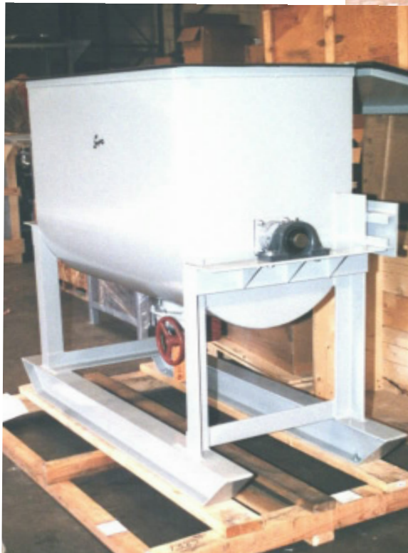
End view of paddle mixer showing non drive end.
