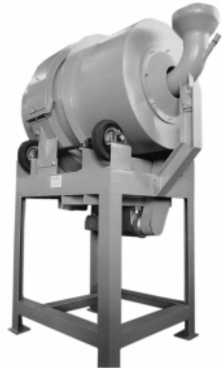
GENERAL ARRANGEMENT DRAWING OF DRUM AMALGAMATION UNIT WITH FEED CHUTE AND MERCURY SEPARATOR OR DISCHARGE CHUTE
