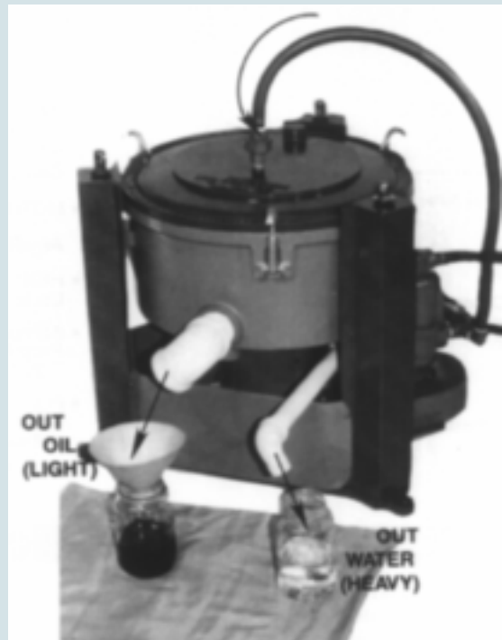
Liquid Liquid Centrifuge Model 1912 Shown Separating Oil From Water
